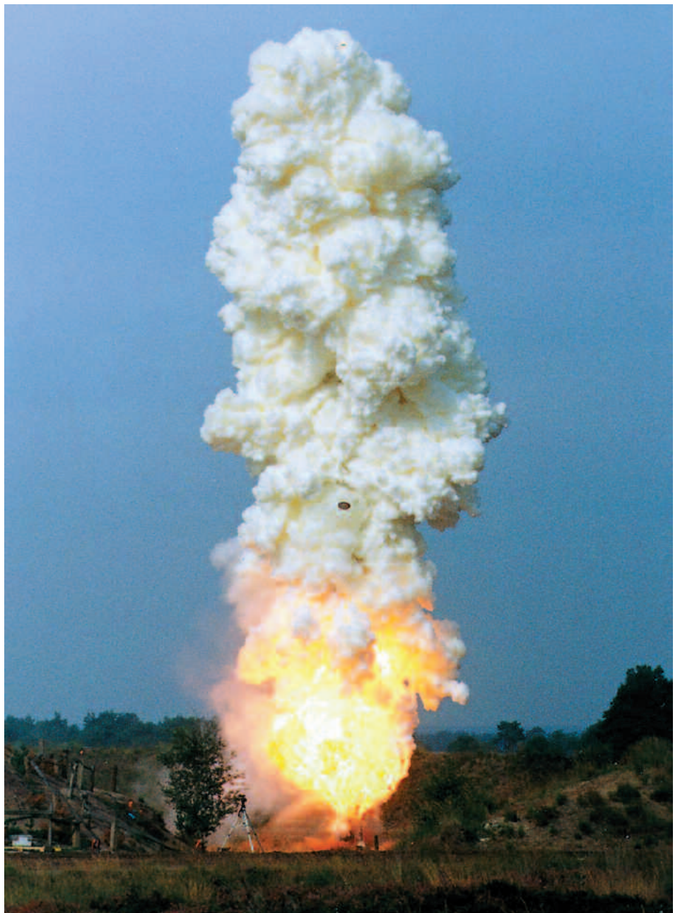
Fire engulfment test of an intermediate bulk container filled with 600 kg of an organic peroxide.
