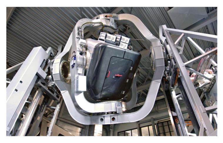
The multi-purpose Desdemona simulator recently installed at TNO will definitely push the limits of motion simulation. Desdemona is a flight and driving simulator, disorientation trainer and advanced research lab, all in one. This simulator - unique to the world - can be used for both research and the simulation of complex situations that may occur during (military) flight, driving or even sailing.
