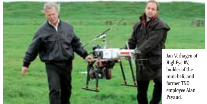
The instrument bank developed by TNO: B/W, RGB and IR cameras and a PC for storing the data, plus a small video camera for flight monitoring.
