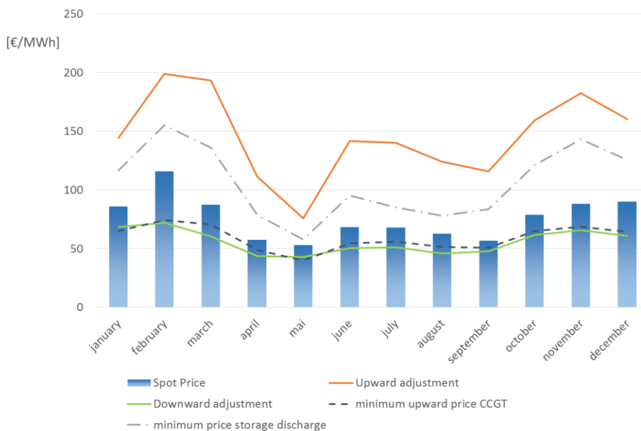
Figure 70: Comparison of 2023 intraday market prices and break even prices for flexible power generation and storage
