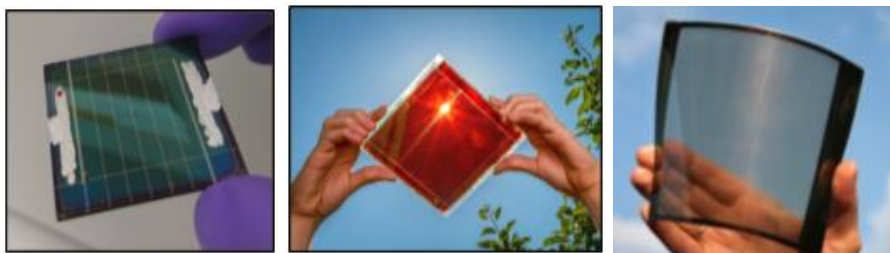
Examples of semi-transparent and see-through thin-film PV products.
