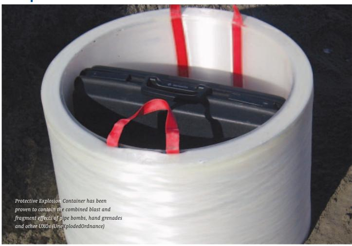
TNO offers a vast range of services and products for public safety. TNO and Futura Composites B.V. developed an Protective Explosion Container, the Episafe. This Episafe has been proven to contain the combined load of blast and fragment effects of pipe bombs, hand grenades and other UXOs (UneXplodedOrdnance). The Episafe redirects the blast upwards and captures the lethal fragments.
