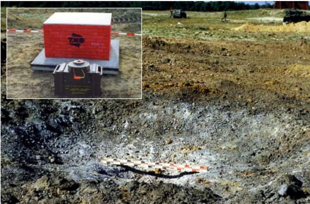
*Small-scale test to investigate the effects of an accidental explosion in ammunition magazines.*
