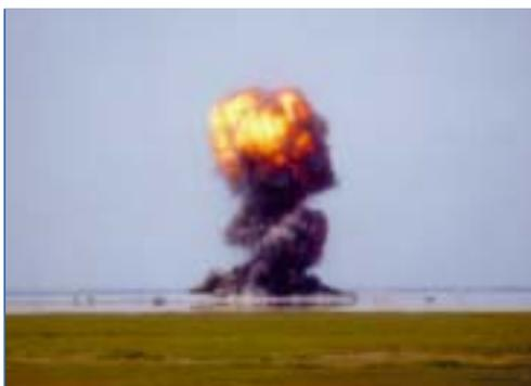
Full-scale test with a net explosives quantity of 1,000 kg (300 mm zoom lens at 1300 metres).
