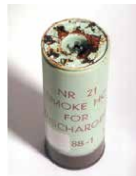
Corrosion on a smoke handgrenade
