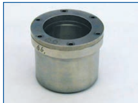
Volume : 70 ml Applicable for 7 and 18 holes grains {comparable to volume of STANAG tube}
