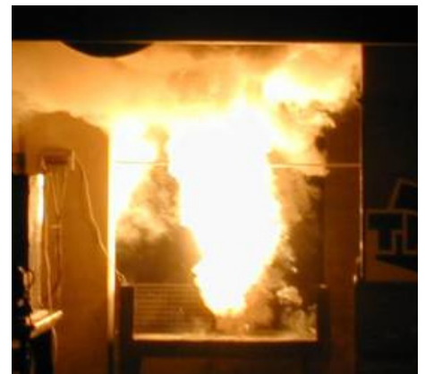
Static tests of an IR-decoy flare at TNO.
