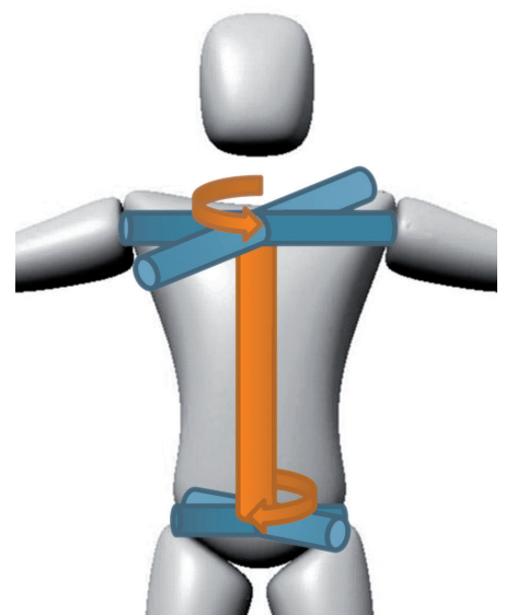
Schematic representation of trunk rotation: each maximum rotation angle between the shoulder and hip line contributes to the summarized trunk rotation angle.
