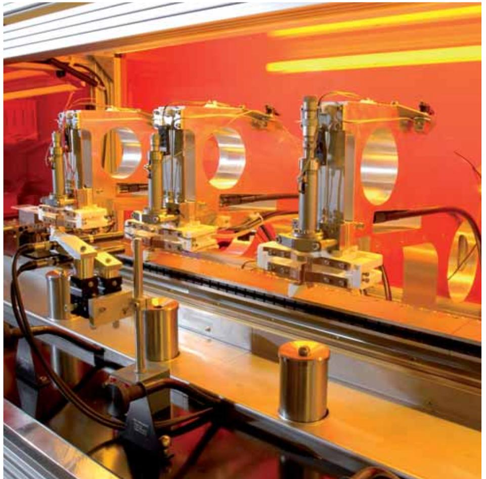
*The print rig with the three print heads developed by TNO*
