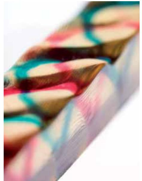
3D graded product made of three high viscous materials
