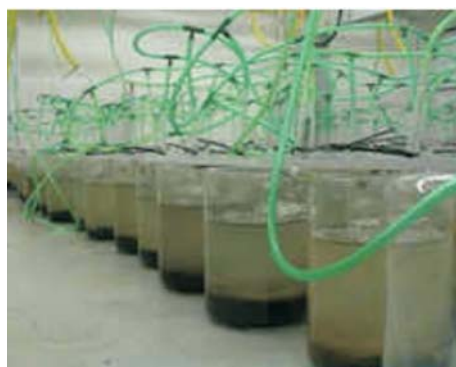
A bioassay is used to determine whether a contaminated sample is harmful to the environment.
