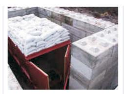
TNO has developed a container for the temporary storage of unexploded ordnance and explosives.
