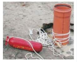
In collaboration with TNO, a civilian firm has developed the 3D-Borehole Radar detection method that enables unexploded ordnance and explosives to be detected at a great depth.
