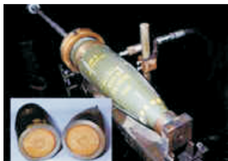
A projectile is cut open and washed out with high pressure water
