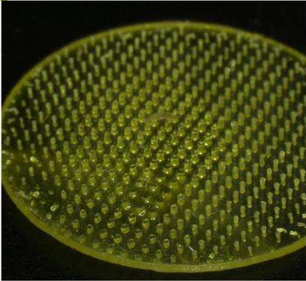
For the gut-on a chip, a surface mimicking the villi of the gut can help to improve the cell differentiation.<sup>1</sup> By using additive manufacturing at TNO EfAM in Eindhoven, a project has started to fabricate these villi-like structures. First a material has been developed suitable for cell adhesion and growth which was successfully tested with Caco2-cells. With this material, micron size features up to ~150µm can be
