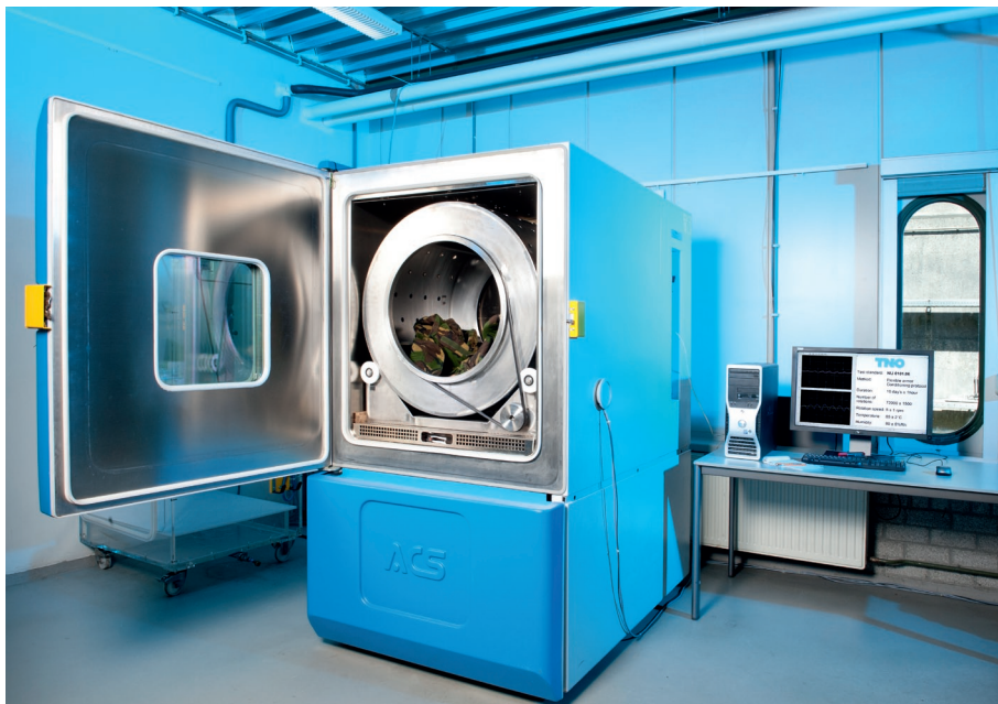
Computer controlled tumbler for the environmental tests
