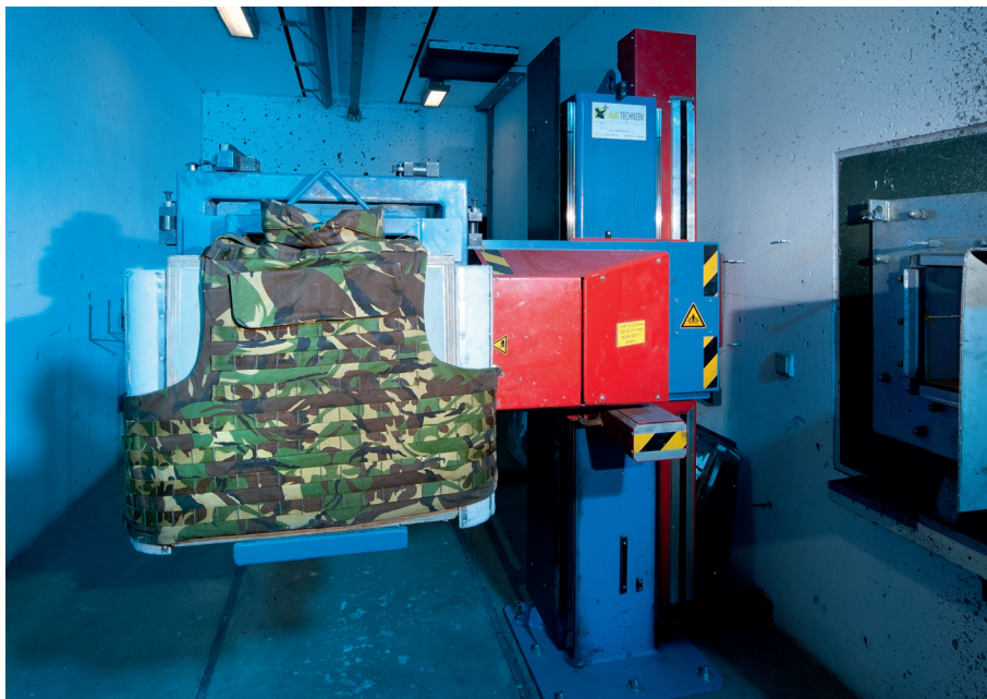
Bulletproof vest fixed in the fully automated test rig
