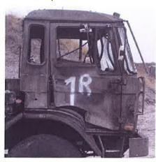
Structural deformation in old truck cabin after a road side IED blast test.
