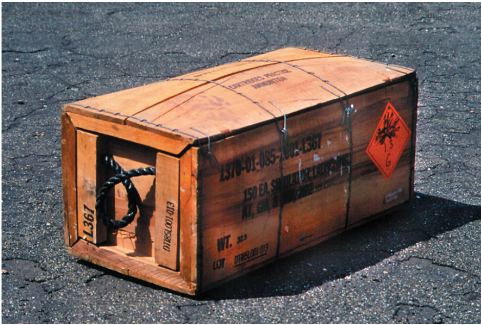
Swelling due to the formation of hydrogen gas.
