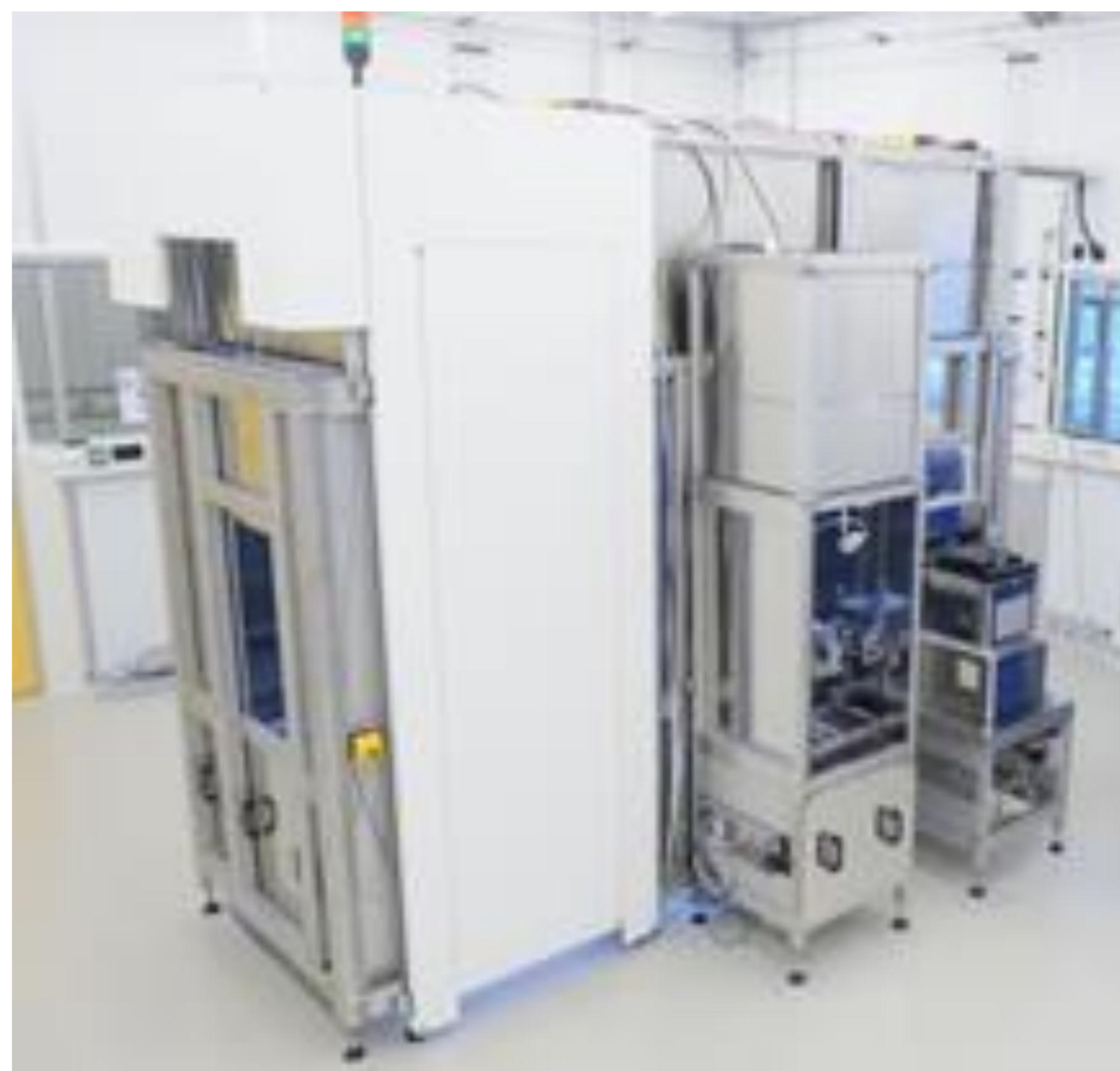
Figure 3: Reticle handler in ICCC cleanroom
