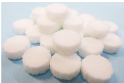
3D printed tablets (round, oval, and donut) produced by means of powder bed printing. (TNO)
