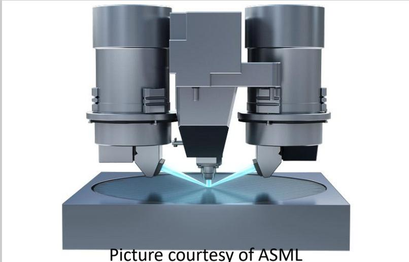
Diffraction from gratings on Si-wafers
