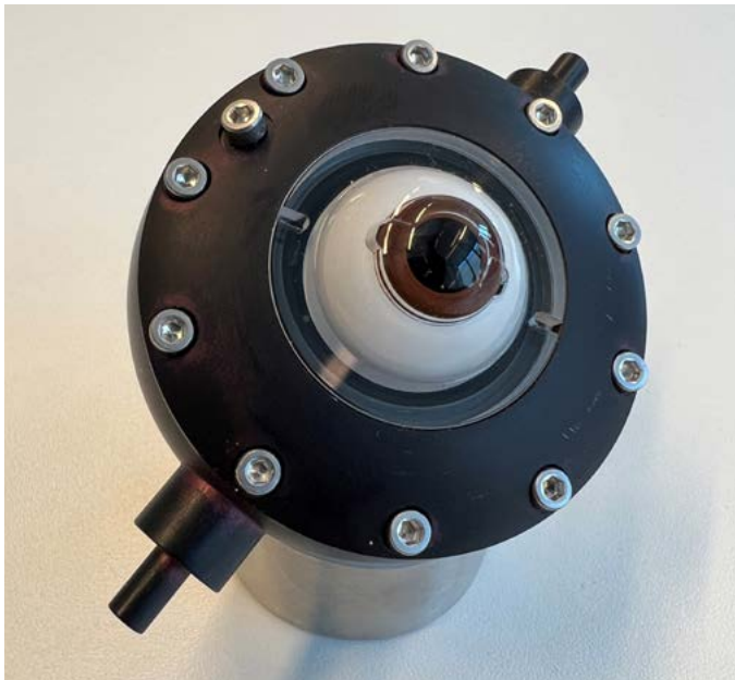
A 3D dynamic Model Eye used for the validation of retinal oximetry devices. A 100µm blood vessel is embedded in a silicone matrix layer with scatterers to simulate the light scattering properties of the retina and choroid.
