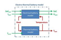
Figure 1 Electro-thermal battery modelling structure
