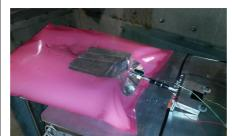
Figure 5 Example of an abuse test with gas analysis
